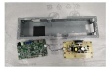
Step.8 Remove connecter cable and separate main board and power board, separate Mylar and shielding
