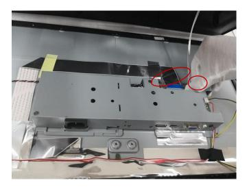
Step.5 Unscrew screws on main shielding and disassemble AL tape
