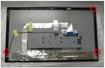
Step10. If with speaker model, assembly speaker on middle frame, and assembly speaker cable on main board. (red and white cable is on left side, yellow and black is on right side.)
