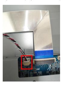
Step6. Insert 30 pin LVDS FFC to main board. Use AL tape to fix. (Tape in blue circle).
