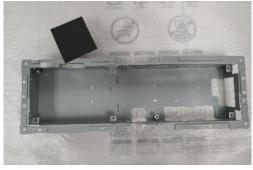
Step.9 Unscrew eleven screws and separate MID FRAME and LCM
