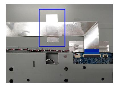
Step7. Tape yellow tape to fix FFC. (Tape in red circle).
