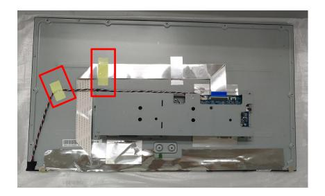
Step8. Assembly middle frame with LCM and fix screw (in red circle)
