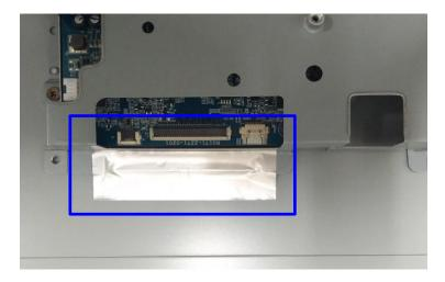
Step5. Insert 6 pin back light WH to panel and main board, use acetate tape to fix. (Tape in red circle).
