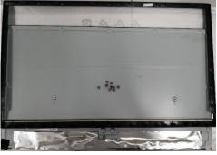
Step.10 Separate gasket and lens from MID frame
