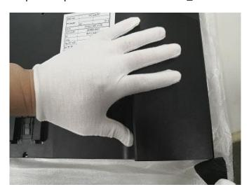
Step 4. Pull up the Rear Cover and pull out all connectors
