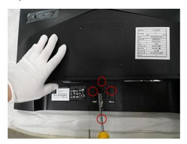
Step.3 Separate hooks between MID\_FRAME and R/C
