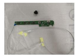
Step.12 Separate wall-mount BKT and display key from rear cover
