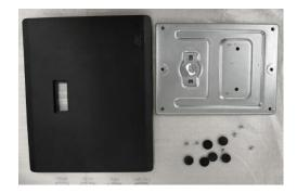
Step 15. Separate back cover from neck, unscrew five screws and separate front cover from hinge assy.
