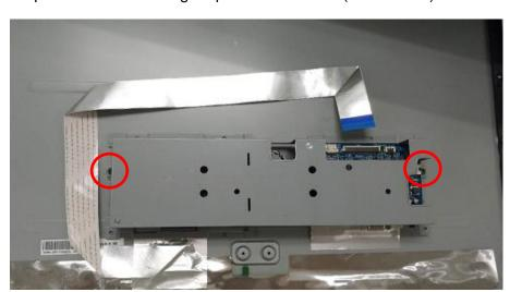
Step4. Use Al tape to fix shielding (tape in blue circle).
